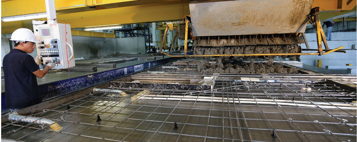
Figure 30. Highly controlled fabrication of precast wall panels. Source: Tekla. Retrieved from: https://www.tekla.com/solutions/precast-fabricators/fabrication .
